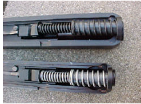
Double recoil spring system of the Model 30 (top) and Model 26 (bottom).
